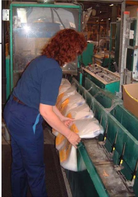
Worksites often have design weaknesses, which might contribute to improper work postures. In certain manual tasks, operators handle produce and packaging material too far away from the body and with twisted torso; in handling details of boxes there are unnecessary loads due to incorrect placing of storage of produce. The storage surface is often a scissor table with a pallet, where the operator places the packed box. The full boxes are often too heavy to handle manually.
