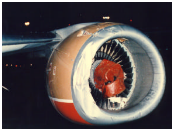
Figure 11 100 Litre Oil Drum Ingested into B737 Aircraft CFM 56 Engine
