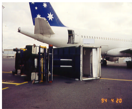
Figure 12 Catering Vehicle Overturned in Impact by Aircraft Under Tow
