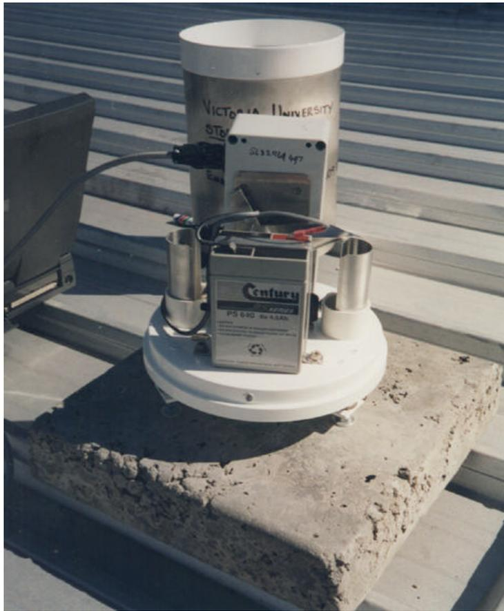
Figure 1: Installation of a pluviometer on a roof of a building
