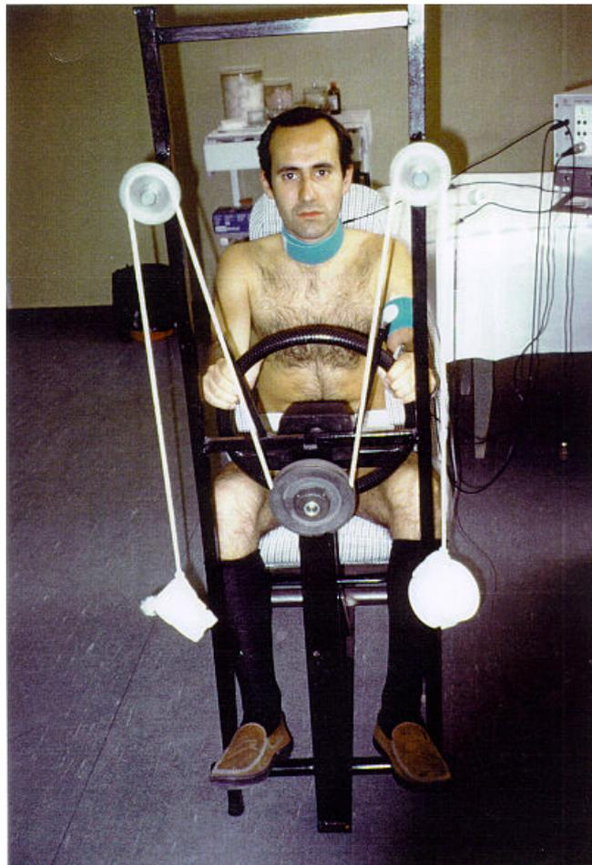
Fig. 1 The simulator which illustrates the system of weights and counterweights connected to the steer.
