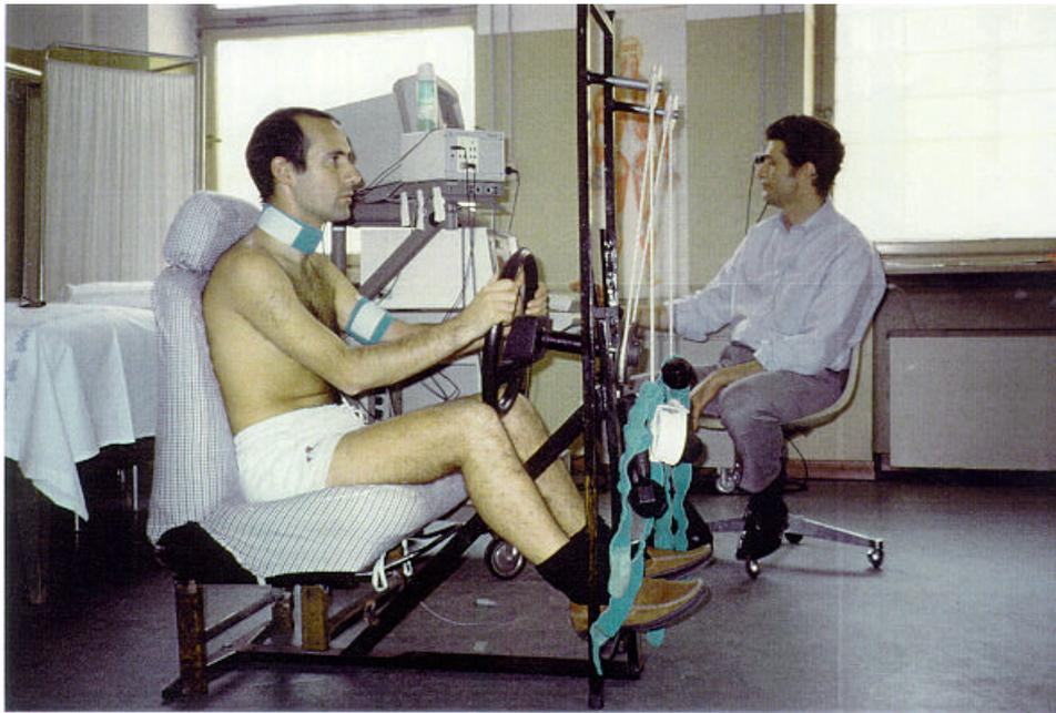
The correct position, with the back of the seat positioned at 25° behind the vertical axis and upper limbs flexed at the elbow in order to achieve a 90° angle between the arm axis and the steer plane.
