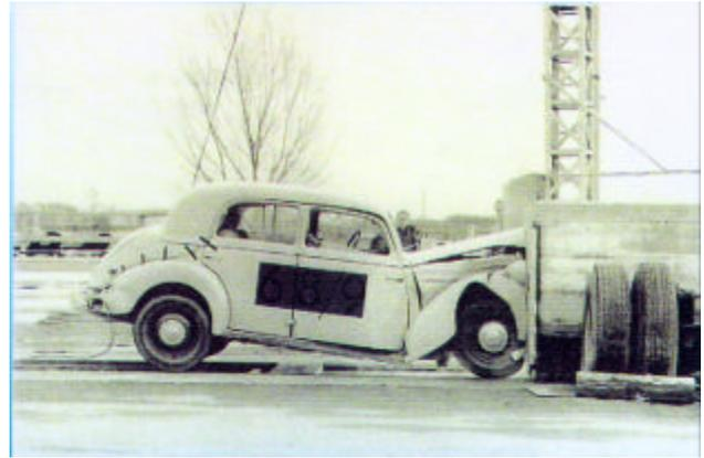
Figure 2 Crash against a rigid barrier with 100% overlap at 50km/h
