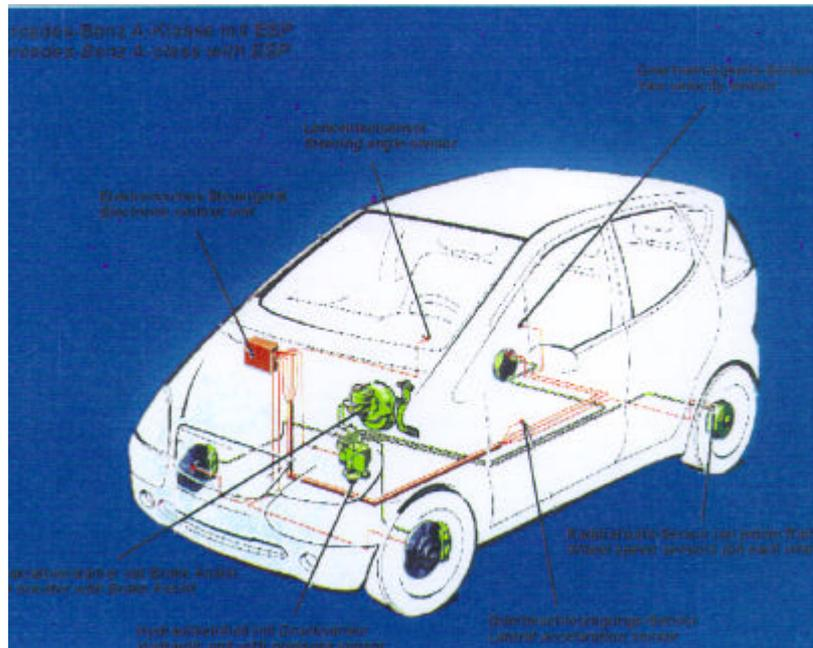
Figure 15 Electronic stability system
