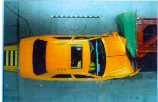
Figure 5 Crash into a deformable barrier with 50% overlap at 60 km/h
