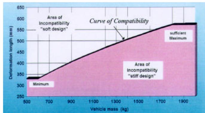
Figure 12 Required dynamic deformation length (Flat barrier impact at 50 km/h)
