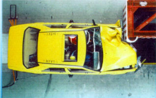
Figure 4 Crash against a rigid barrier with 40% overlap at 55 km/h
