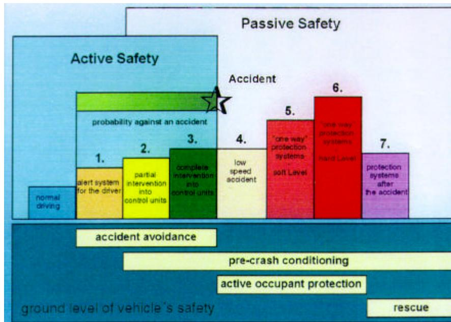
Figure 16 Phases of occupant protection
