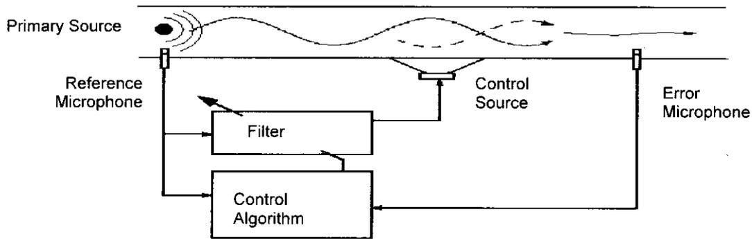
Figure 5. Feedforward Control
