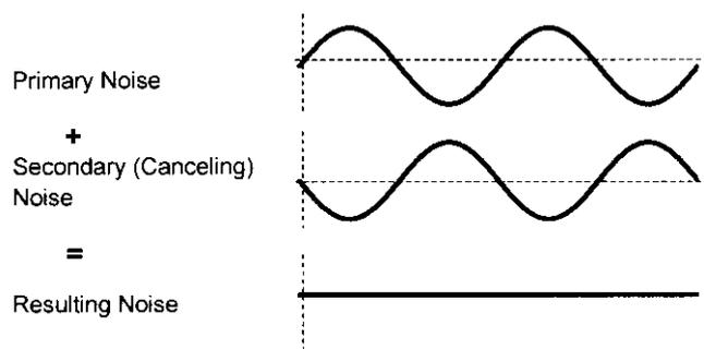
Figure 3. The principle of Active Noise Control
