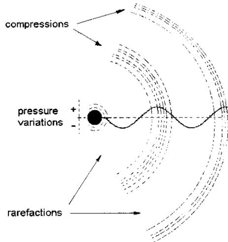
Figure 2. Transport of sound waves, from a vibrating body
