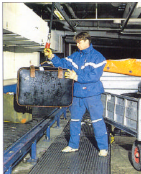
Figure 10 - The AirGro “ErGoBag” Mechanical Assistance Device
