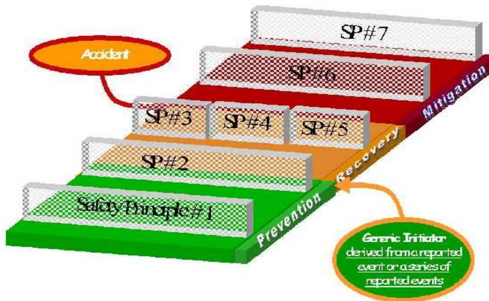
Figure 7 Safety Architecture (i.e. combinations of Safety Principles) associated with a Generic Initiator
